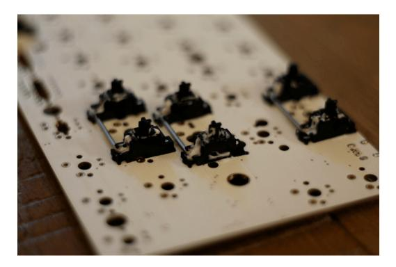
All parts of the stabilizers that move have grease on them. This prevents the parts from clicking together and echo as well as ensure smooth vertical travel.
