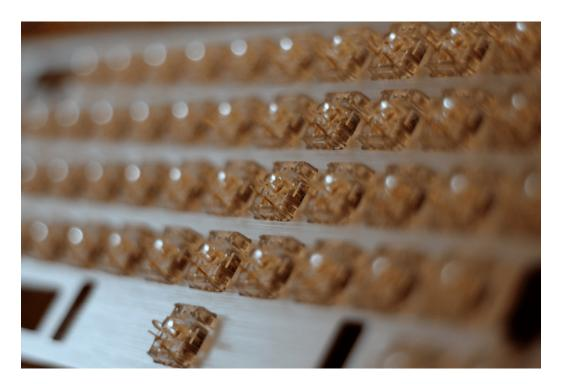
For the longer open parts of the plate that allow for multiple positions, we leave the switches out until we can fit them in with the plate before soldering to ensure they are lined up correctly.
