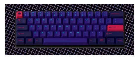
This set is manufactured in Germany by an electronic design company called <u>GMK</u>. The material used is <u>ABS</u>, an impact-resistant plastic. The legends are not printed with ink: rather they are molded into the plastic in a process called double-shot molding <sup>8</sup>.
