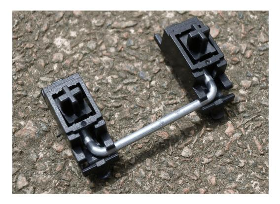
Cherry, another German electronics manufacturer, makes high-quality stabilizers that screw into the PCB in lieu of clipping into it. This gives the stabilizer added stability in addition to its intended purpose. Applying a lubricant like dielectric grease can help reduce the added friction stabilizers cause during the keypress.
