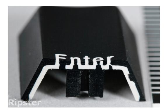
This means the legends will never wear down. The thicker plastic used in the molding process also means the keys are more rigid, which provides a more precise feeling typing experience. The plastic is also textured, which makes it preferable to type on.
