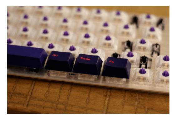
Once the switches are all pressed into the PCB, we can carefully begin to solder all of them into their respective places. This build does not include LEDs, but they would be soldered in this stage too if it included some.
