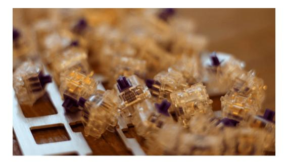
The Zealio switches support PCB mounting; they do not need a plate. They have additional legs that allow them to sit flush with the PCB:
