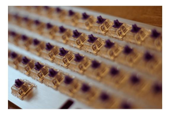
Note that the KBD 660 PCB orients the switches upside down, so the underside of the plate should look like this:
